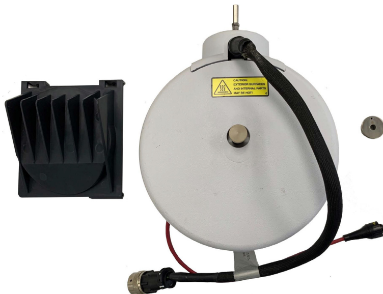
Figure 6. APCI cover, ion source, and spray shield
