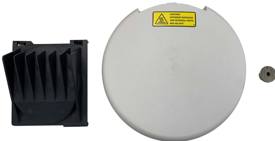
Figure 4. ESI cover, ion source, and spray shield
