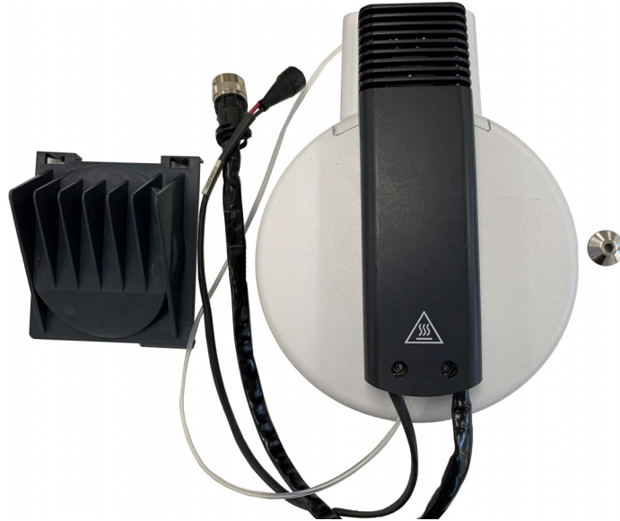
Figure 5. AJS cover, ion source, and spray shield
